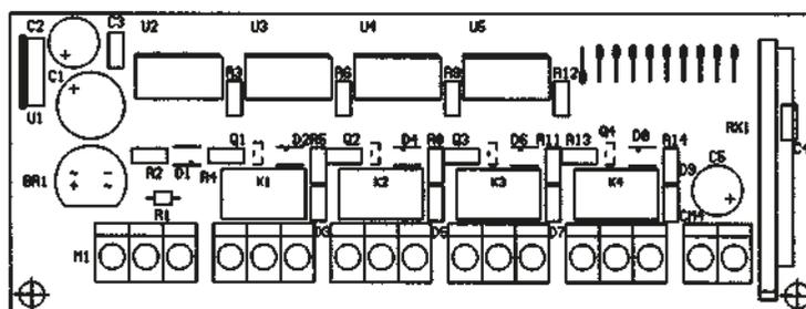
RICEVITORE RADIO DIP SWITCH DA 1 A 4 CANALI
